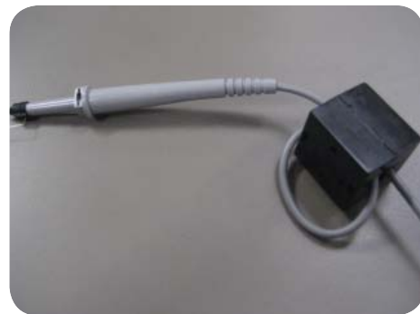
Figure 7-1. Using a ferrite core on the probe cable may help improve probing accuracy
