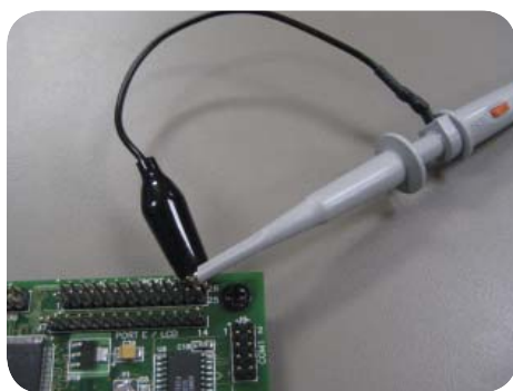
Figure 6-1. Connect both probe tips to the ground and see if any signals appear on the screen.
