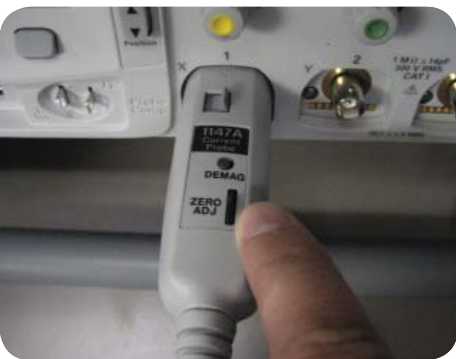
Figure 4-2. To improve current probe’s accuracy remove magnetism and DC offset
