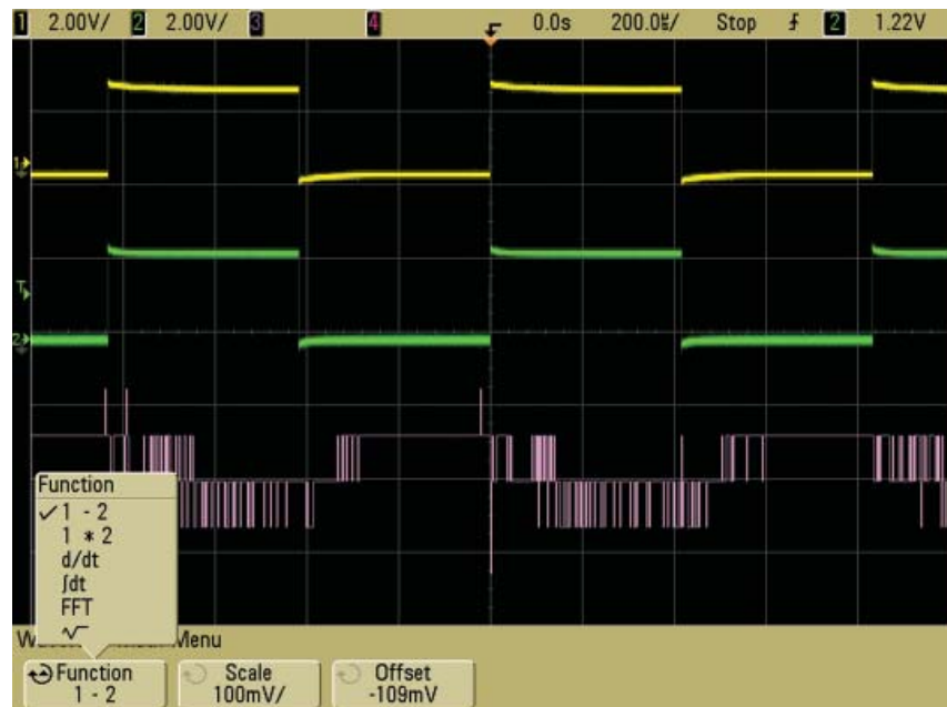
Figure 5-2. As a sanity check, double probe the same signal and see what the "A-B" looks like.
